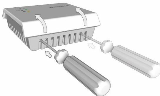
Continue to move the upper part with all the electronics until it is separated from the lower part.
