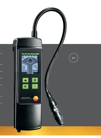
The testo 316-4 (Set 1) is a fast and reliable leakage detector for all common refrigerants. The sensor is permanently monitored and shows malfunctions or contamination in the display. The use of test leaks is thus superfluous. If dirty, the sensor can simply be cleaned, and is immediately ready for use again.
